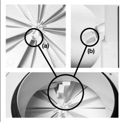
Once in place, locate the fascia over the base unit ensuring that the placement lug of the back plate (a) lines up with the receptor void on the perimeter of the fascia (b).
