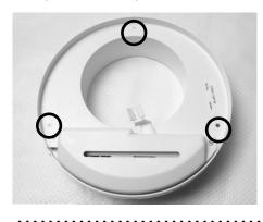
Align the fascia notch (a) on the back of the fascia, with the base unit control arm (b). This ensures that the humidity sensor controls the opening and closing of the grille.
